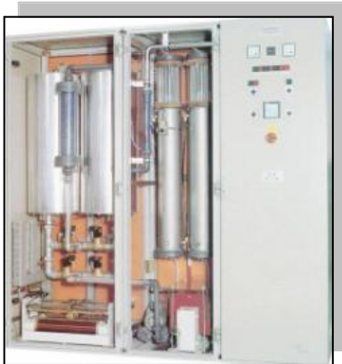
A corona discharge generator capable of delivering 80g/hr O 3 continuously. This unit uses outside air and does not require the use of bottled oxygen to generate ozone (O 3 ).
